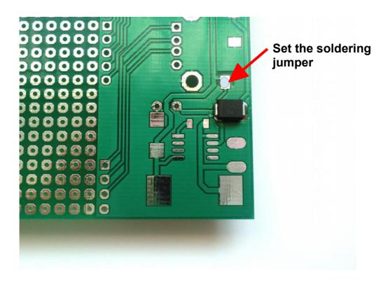
Perform the next steps only if you have the standard kit (includes the parts of the voltage regulator and USB socket). Otherwise continue with step 16.
