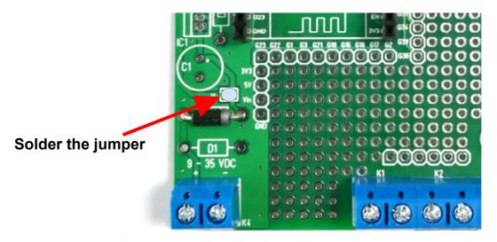
Perform the next steps only if you have the standard kit (includes the parts of the voltage regulator and USB socket). Otherwise continue with step 12.
