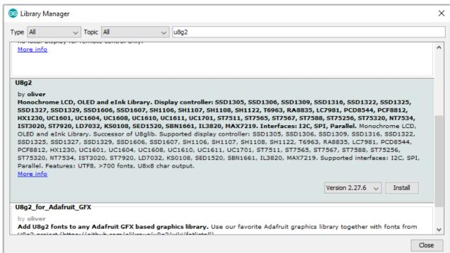
Click the Install button. After some seconds "INSTALLED" will be displayed.
