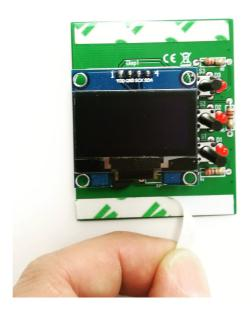
Glue the shield into the top shell:
