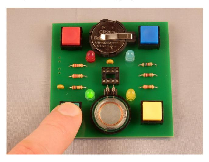
If one or more LEDs not shine, you have to check the assembly direction (cathode/anode) of these LEDs. Furthermore check the soldering of the LED, corresponding resistor and button.
