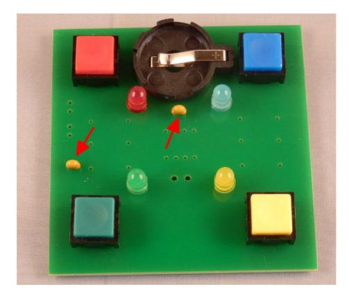
5.) assemble the 120 Ohm resistor (R6)
