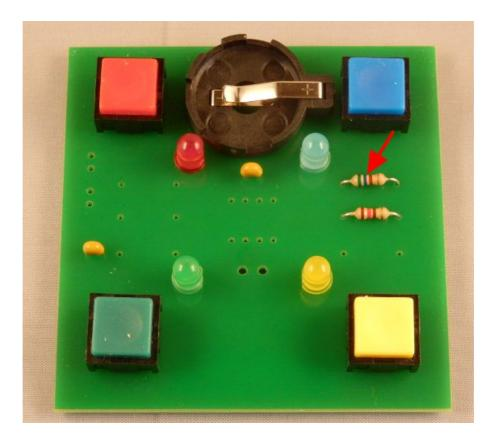
7.) Assemble the 10K resistor (R5)
