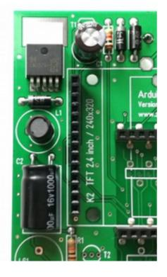
10.) Place and solder the transistor T2 (BC547)
