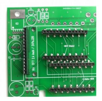
4.) Place and solder the schottky diodes D1, D2 & D3
