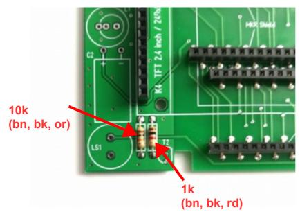
5.) Place and solder the resistors R2 and R3
