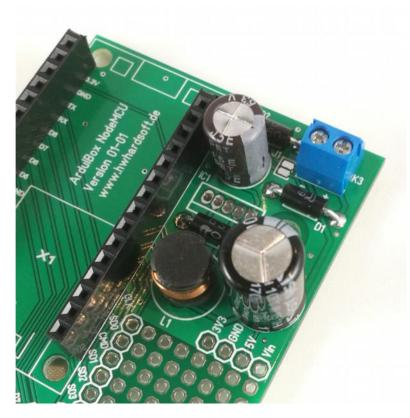
13.) Assemble voltage regulator IC1
