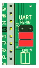
For use with an **MKR 485 shield:** GPIO15 is connected with RX (D13) GPIO 14 is connected with TX (D14)
