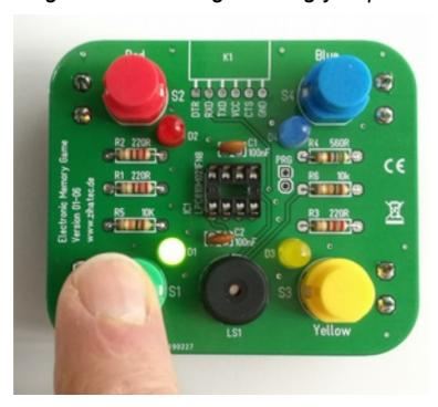
If one or more LEDs not shine, you have to check the assembly direction (cathode/anode) of these LEDs. Furthermore check the soldering of the LED, corresponding resistor and button.
